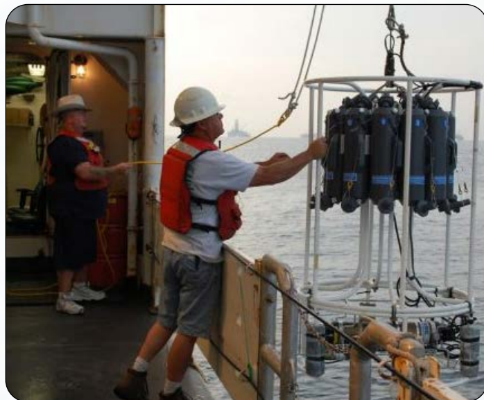
Figure 2: CTD rosette illustrating sampling bottles (top of structure) and submersible sensors (bottom of structure).
