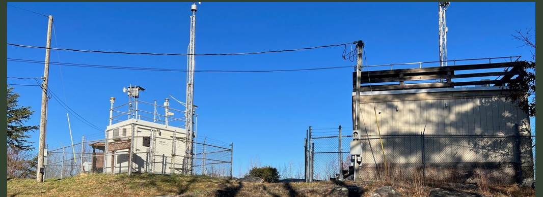
Look Rock CASTNET site (GRS420, TN) co-located with IMPROVE and Atmospheric Science and Chemistry Measurement Network (ASCENT). ASCENT will provide high-time resolution measurements of black/brown carbon, PM speciation, metals and PM sizes at 3 CASTNET sites.
