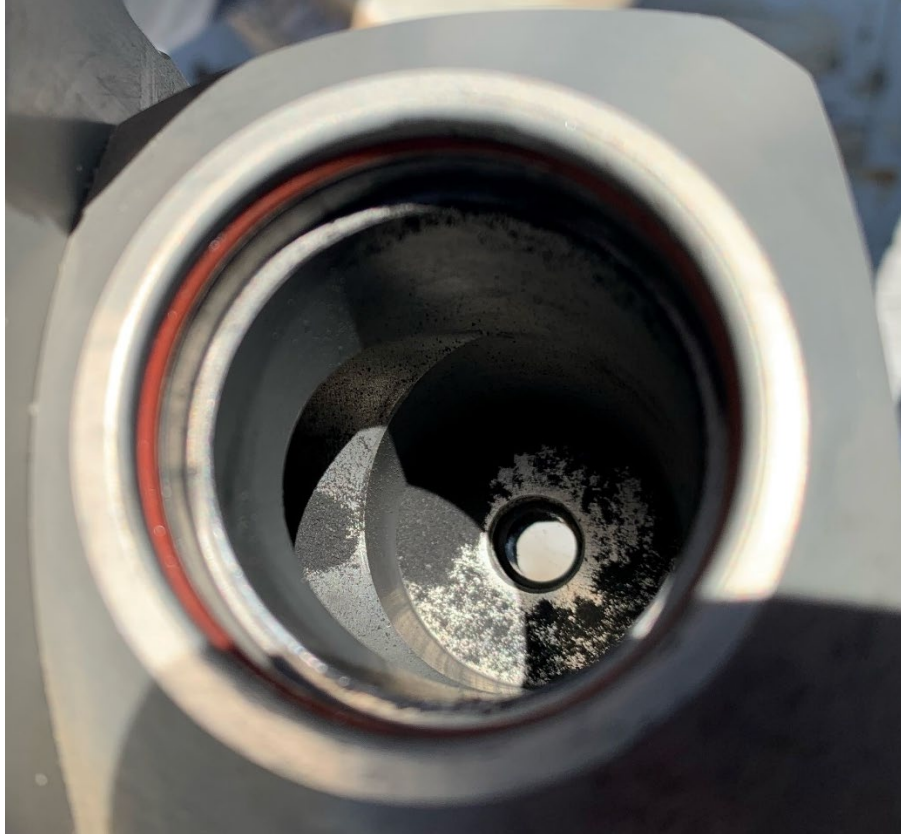
Figure 6. Photo of URG 3000N Inlet Tee with “black dust” buildup (taken July 13, 2023).
