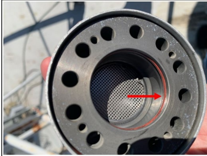
Figure 7. Photo of Inlet Cap removed from Downtube with o-ring indicated by red arrow (taken July 13, 2023).
