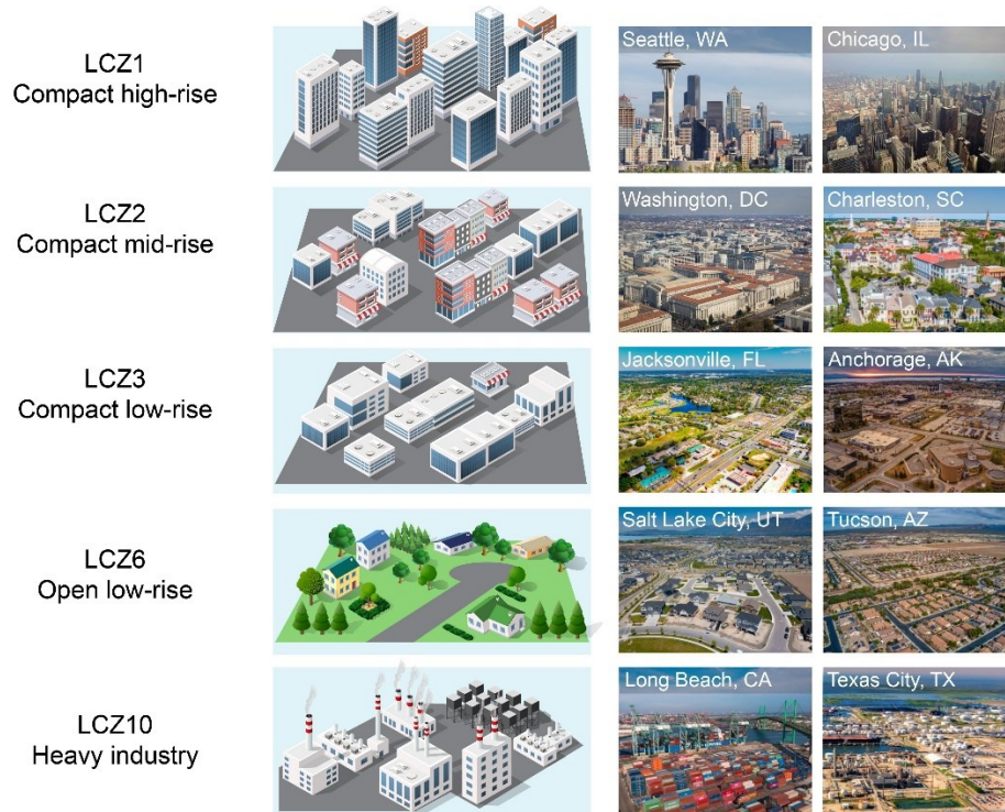
Figure 2: Illustrative land-use classifications of local climate zones (LCZs). Urban areas of the Midlands are most commonly LCZ6, with some exceptions including downtowns of certain Midlands municipalities. Figure copied from the National Climate Assessment, Chapter 12. 3
