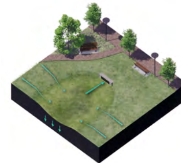
■ ■ Dry Detention Pond
