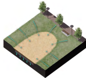
■ ■ Surface Sand Filters
