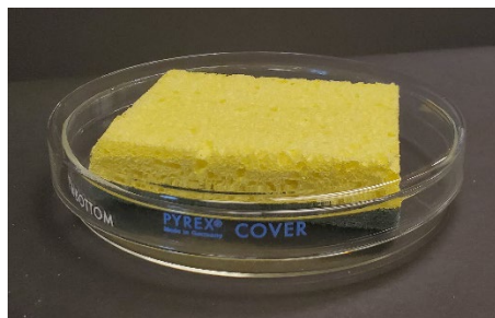
Figure 3. One sponge, pre-cleaned and cut to fit snugly in abrasion tester sponge box, shown in 150 mm glass Petri dish prepared for sterilization.
