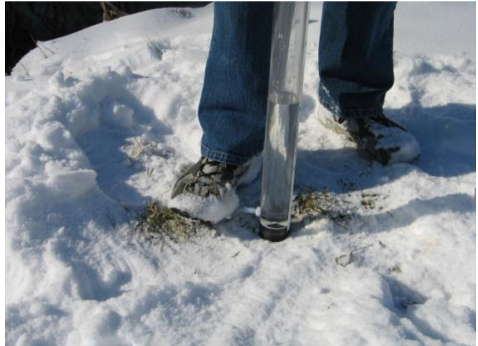
Figure 2: Releasing water until the disk is just visible.
