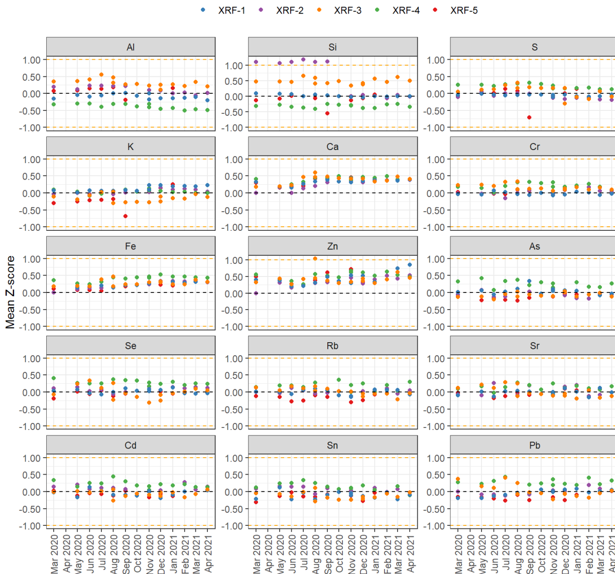
Figure 4.2-3: Inter-instrument comparison by z-score of monthly reanalysis sample set. The orange dashed lines indicate the mean z-score acceptance criteria of \pm 1 . Note there is no result for April 2020 due to the pandemic related shutdown.
