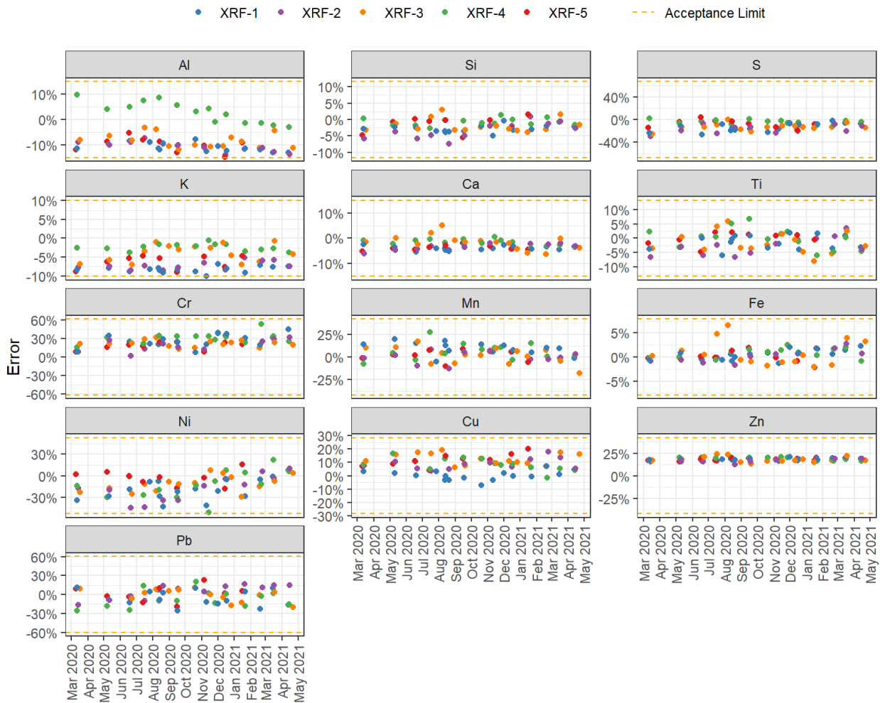
Figure 4.2-4: Error of each EDXRF instrument from the NIST SRM 2783 standard run monthly for the analysis period 3/12/2020 through 4/21/2021.
