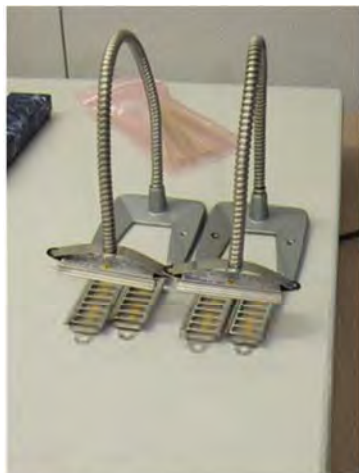
Figure 9.4: ^{210}\text{Po} Anti-static strips & gooseneck holders
