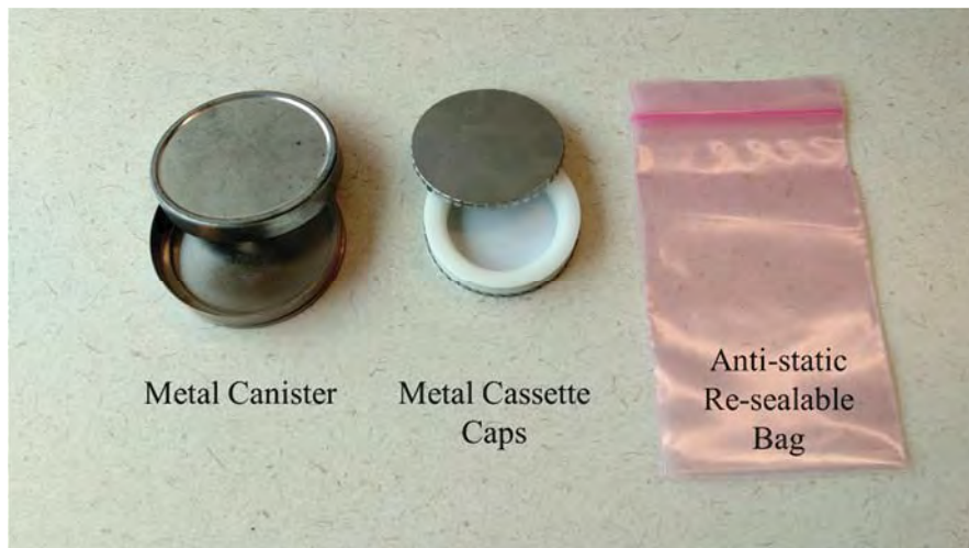
Figure 4.2 Example equipment for transporting filter cassettes
