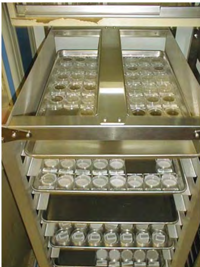
Figure 10.1 Filters equilibrating on conditioning trays
