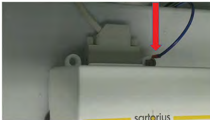
Figure 9.1 Grounding screw on microbalance
