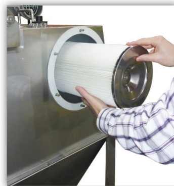
Remove filter through side access plate.
