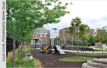
USEPA Louis Cook, Philadelphia Water Dept. A porous play surface made from recycled tires is surrounded by rain gardens and trees.
