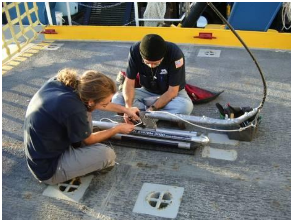
Figure 11. Picture of Klein tow fish attached to electronic cable on OSV Bold stern
