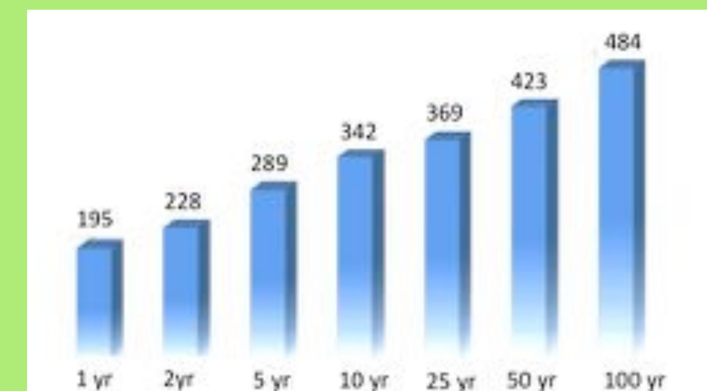
Fig. 4 Gallons (x 1000) of Runoff accrued from PV canopy in 24 hr for storms recurring at various intervals.
